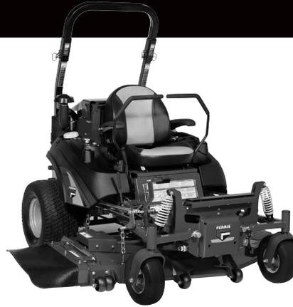
**TYPE:** Mid mount, zero turn, twin stick steering rider with four-wheel suspension
