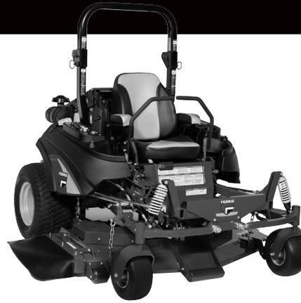
**TYPE:** Mid mount, zero turn, twin stick steering rider with four-wheel suspension
